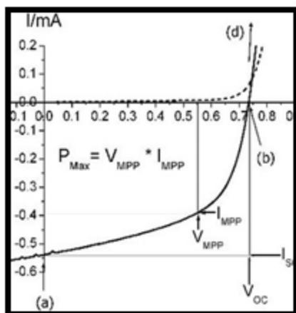
Figure 1. Shown below, are a solar cell’s typical V-I characteristics.
