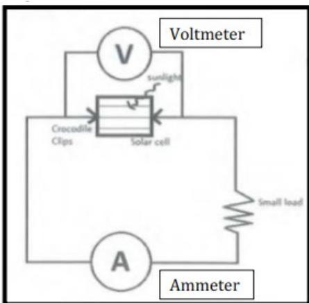
Figure 2. Diagram of the circuit.
