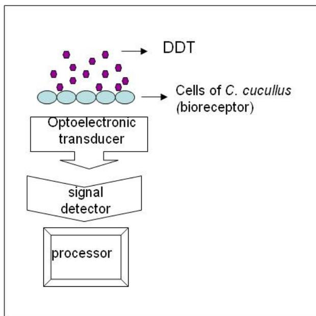
**Figure 9.** Diagram of the optoelectronic whole-cell biosensor.
