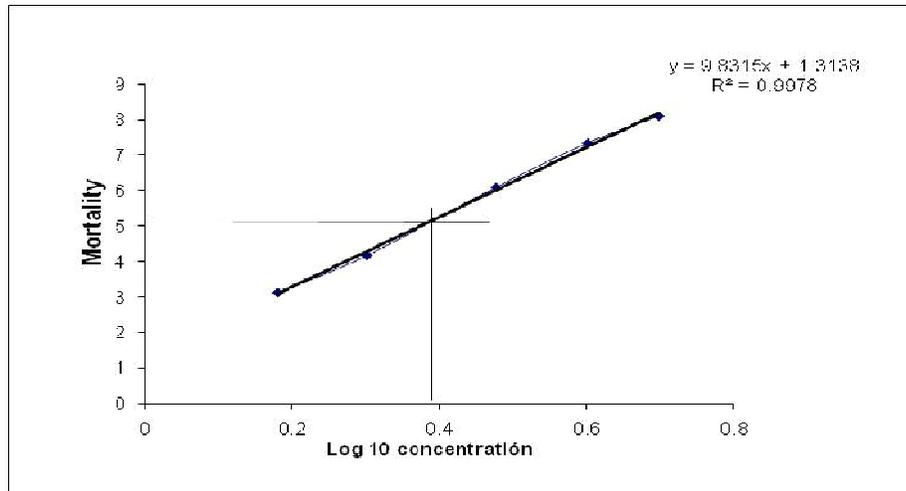
**Figure 5.** Result of the Probit analysis for calculating the  $LC_{50}$  of DDT on *C. cucullus*. The  $LC_{50}$  was  $6.68 \times 10^{-6}$  M DDT after an exposure time of 1 hour
