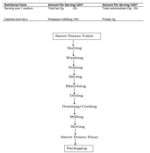
Figure 1. The flow chart for the production of unfermented sweet potato
