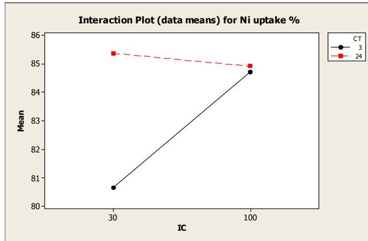
Figure 4 The Interaction plot for Nickel uptake in petroleum wastewater
