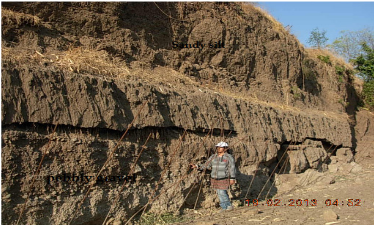
Fig2. Photograph of Sandy Silt – non Calcified on right bank of Sindphana river at Nathapur. The photo facing east.
