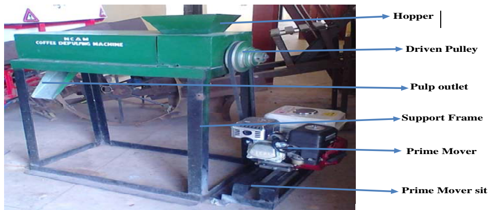
Figure 6. NCAM Coffee Depulping Machine
