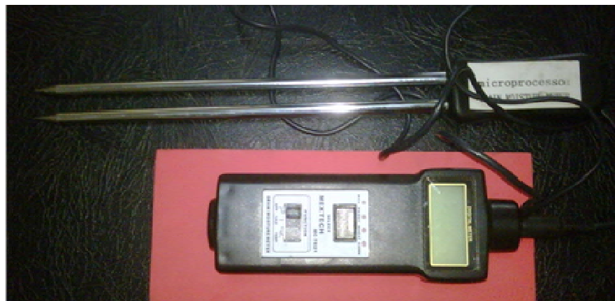
Figure 4. Universal Moisture Sensor
