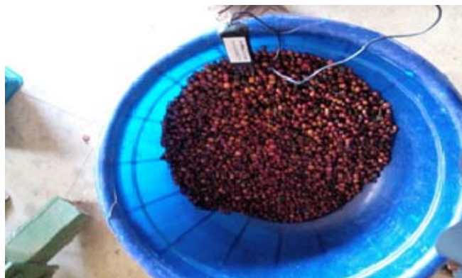
Figure 5. Berry Moisture Content determination using the Universal Moisture Sensor
