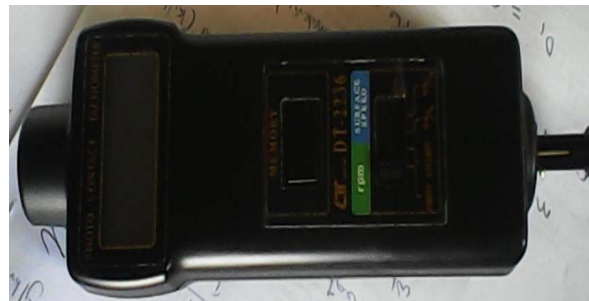
Figure 2. Speed measuring contact Tachometer
