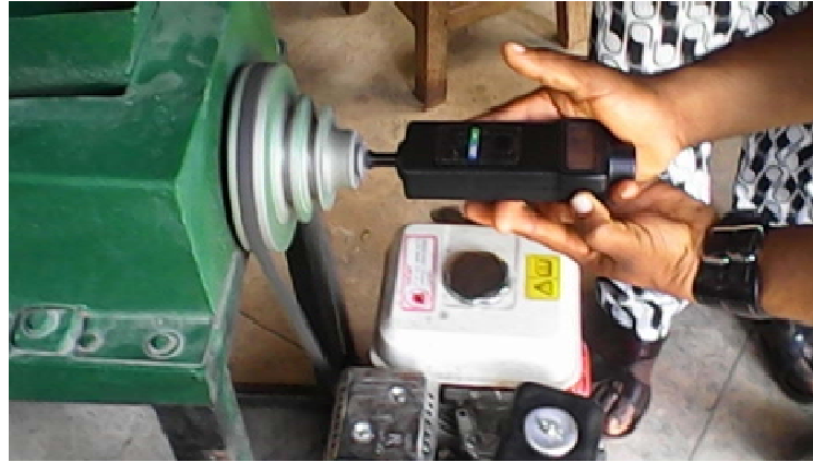
Figure 3. Operating speed measurement using a contact tachometer
