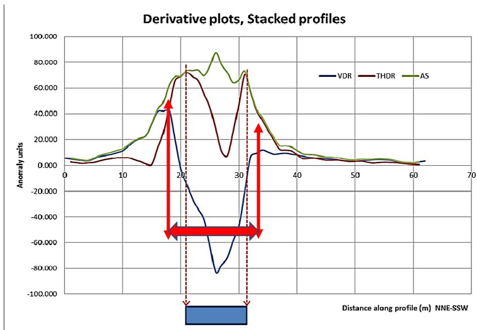
Figure 13. Estimate of width of dyke from derivatives anomalies. Width = 10m and 16m
