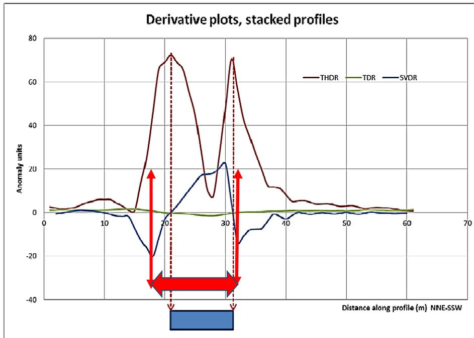
Figure 14. Estimate of width of dyke from derivatives anomalies. Width = 10m and 15m
