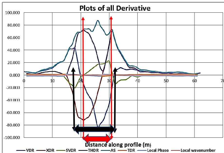
Figure 15. Plots of all Derivatives, Estimated Dyke Width = 10m and 15m
