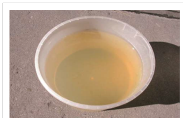
Figure 1: Stained tap water sourced in an apartment
