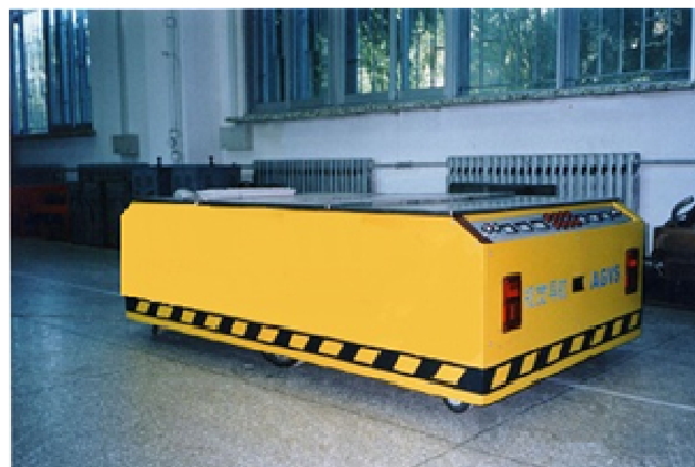
Figure 9. V-AGV experimental platform
