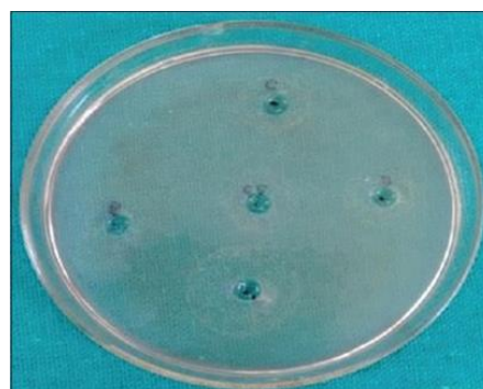
Figure 5. Four hand sanitizers were introduced into each of the 4 wells and central well filled with sterile water.
