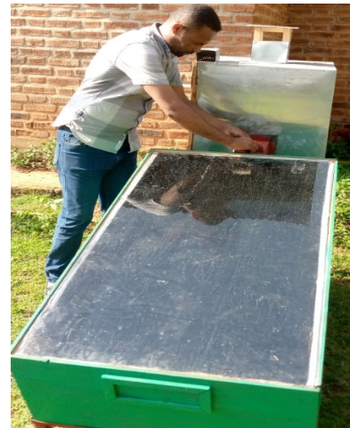
Figure 2. Hot air flow controller device adjustment and reading.
