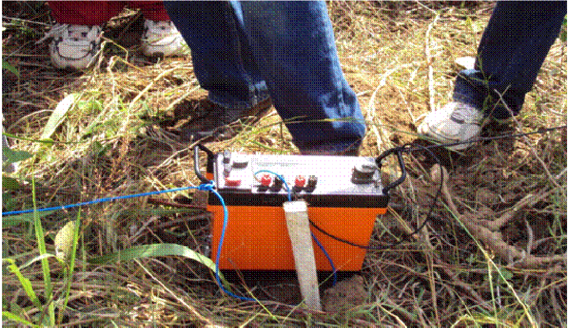
Figure 7. The versatile ABEM SAS 4000 – High resolution resistivity meter. Positioned at probe point.
