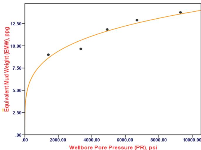
Figure 4.1: Relationship between equivalent mud weight and Wellbore pore pressure on the equivalent mud weight window log while drilling.
