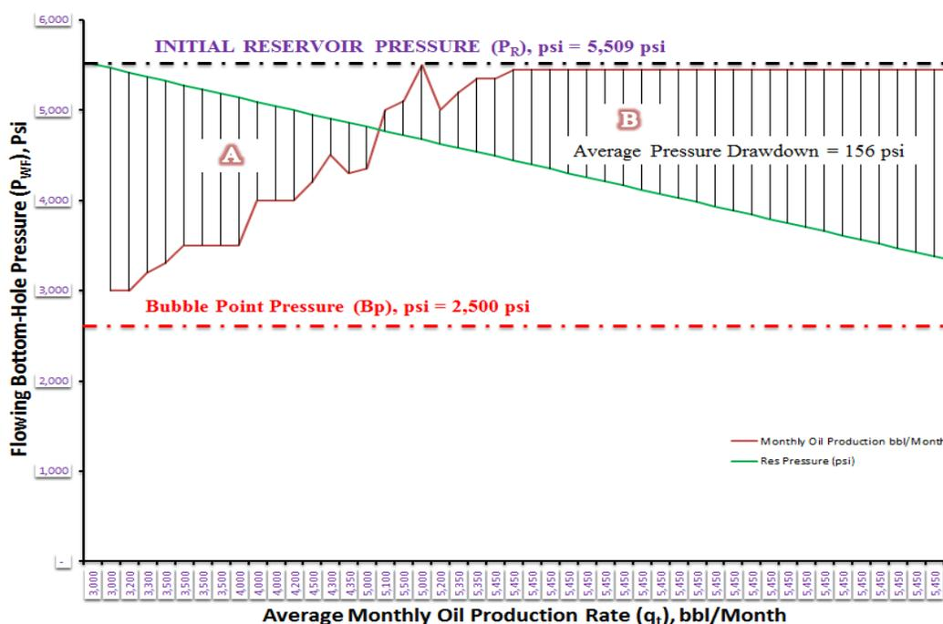
**Figure 4.6:** Flow pattern of oil at the SST4 wellbore bottom-hole as the reservoir pressure undergoes pressure drawdown
