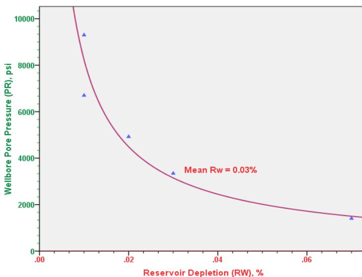
**Figure 4.4:** Relationship between the wellbore pore pressure and Reservoir depletion experienced in the wellbore.
