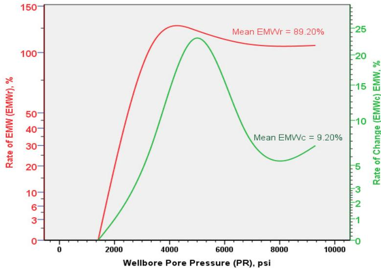
Figure 4.3: Relationship between equivalent mud weight's rates and rate of changes applied on the pore pressure while drilling.
