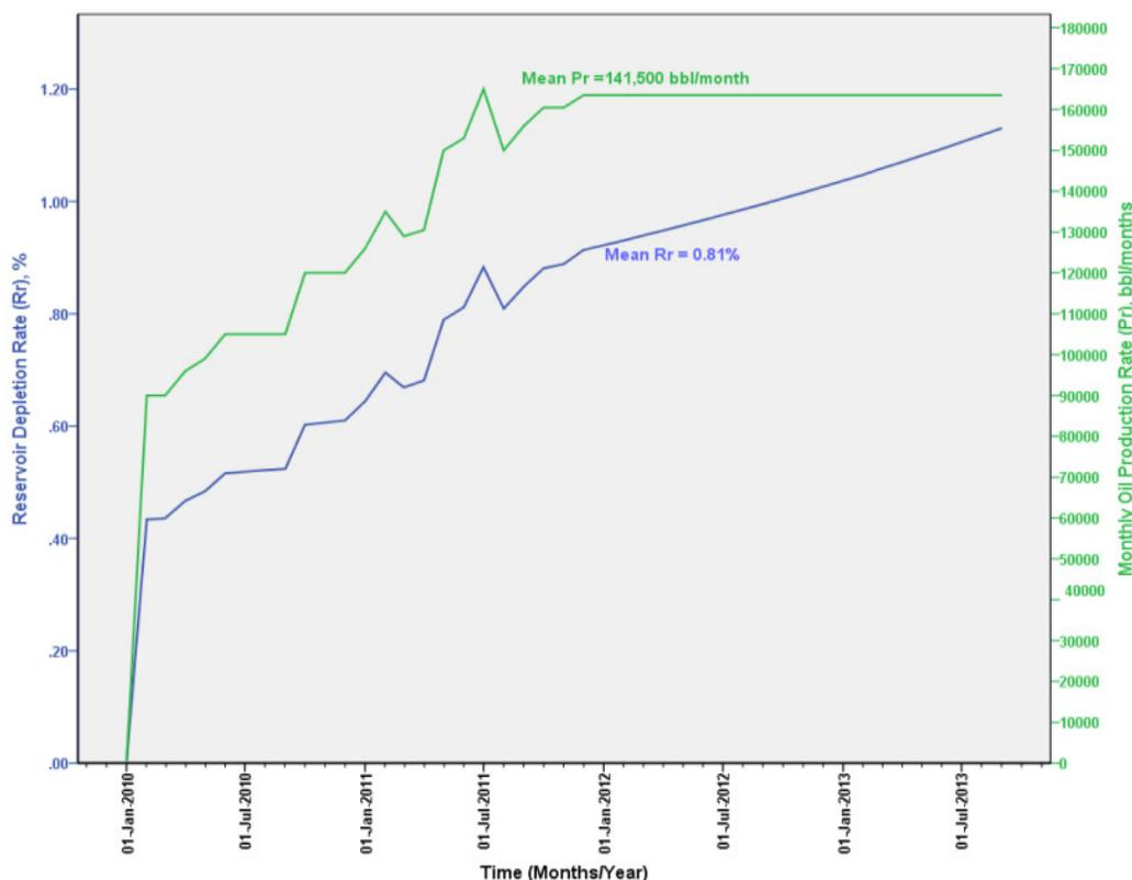
**Figure 4.7:** Mean monthly oil production rate and degree of reservoir depletion at the SST4 wellbore bottom-hole.
