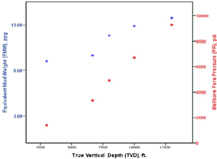
Figure 4.2: The trajectory of EMW and PR while drilling at various measuring depths.
