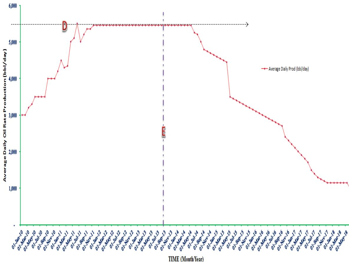
**Figure 4.5:** Monthly Oil rate production at the single well SST4 with solution gas drive mechanism for oil produced between January 2010 and September 2013
