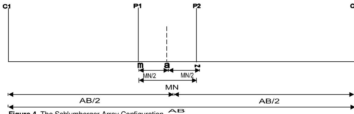
**Figure 4.** The Schlumberger Array Configuration.
