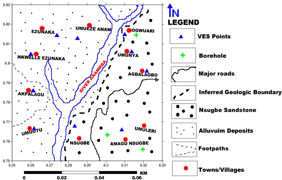
**Figure 3.** Geologic map of the study area showing VES and Borehole locations
