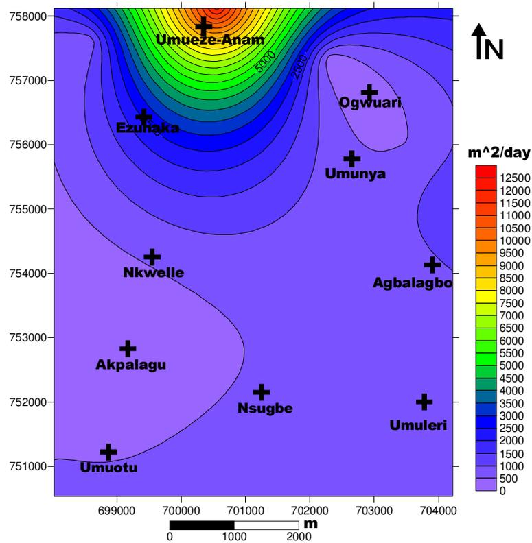
Figure 9. Aquifer Transmissivity Map of the Study Area.
