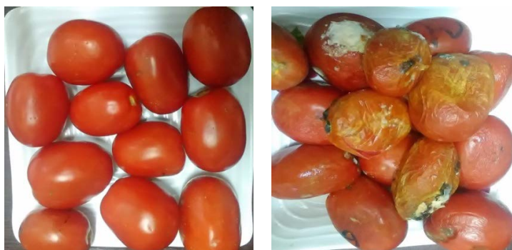
Figure 7: Tomato stored under PIP refrigerator (A) and RA (B) for 15 days.
