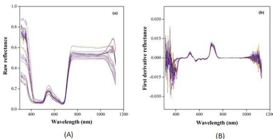
**Figure 2.** (A) Original reflectance of 21 rice leaf samples; (B) First derivative reflectance of 21 rice leaf samples.
