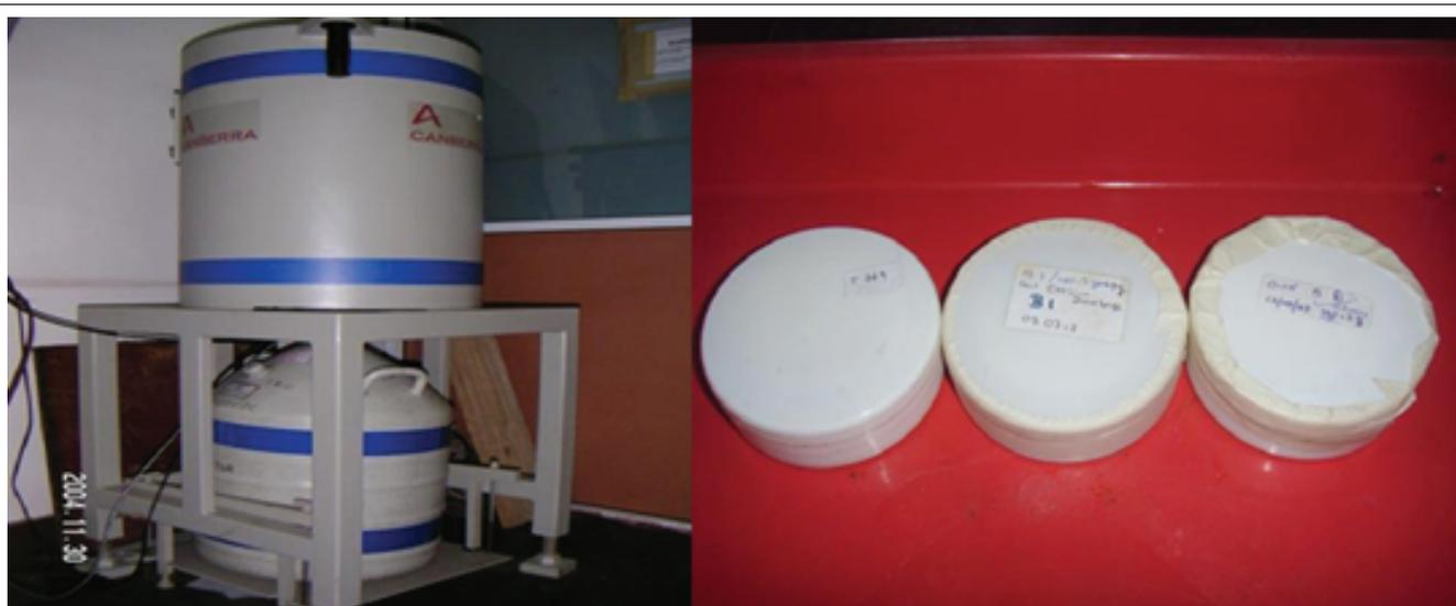
Figure 5: HPGe detector and containers used for analysis
