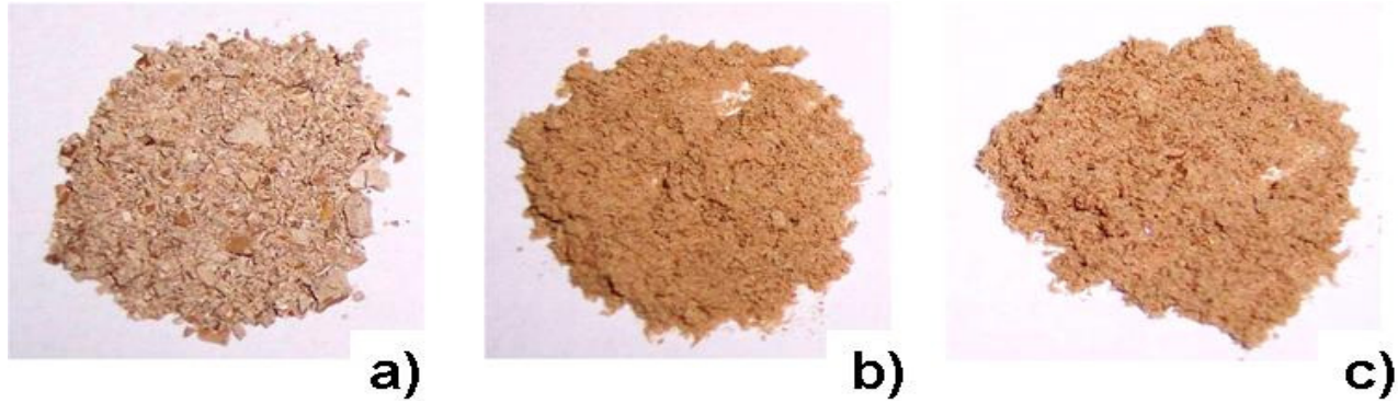
Figure 1. Standard lyophilized material of fructosyltransferase from Rhodotorula sp. LEB-V10: a) without dilution (lyophilized cake with A_w = 0.187 \pm 0.001 and with greater resistance to crushing and dissolution), b) diluted to 1:2 (v/v) (lyophilized with A_w = 0.192 \pm 0.004 , fine powder aspect and fast dissolution) and c) diluted to 1:6 (v/v) (lyophilized with A_w = 0.276 \pm 0.001 , lighter coloration, very fine uniform powder, easy dissolution). The dilutions were achieved in sodium acetate buffer (50 mM and pH 4.5).
