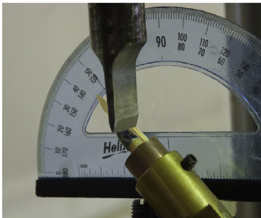
Figure 1. A mounted specimen positioned at 135 0 angle in a custom made holding grip used in the Universal testing machine (MTS 858; MTS Systems Corp, Eden Prairie, Minn) employed for fracture resistance testing.
