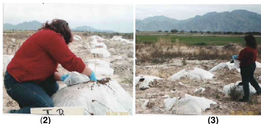
Figure 2 and 3. Taking of samples at different depths for laboratory analysis (2) and temperatures at different points (3) in the pails.
