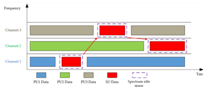
Figure 6. Functional diagram of cognitive radio.
