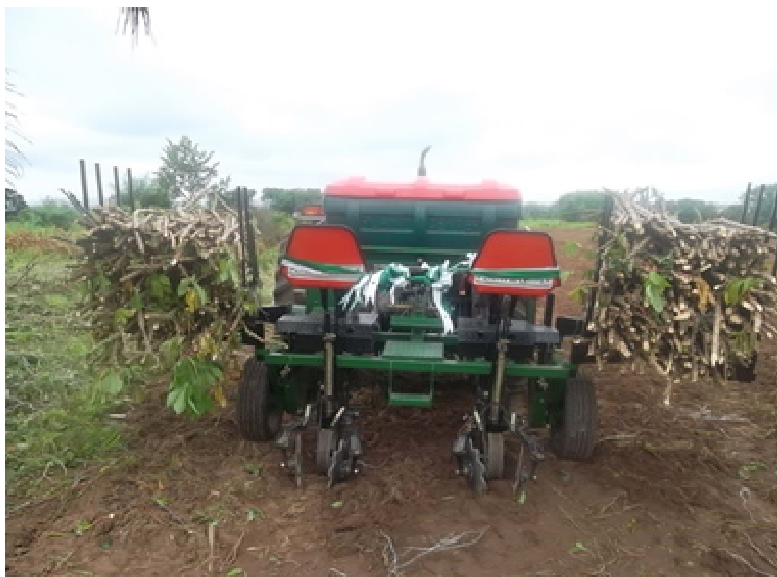
Figure 1: 2 row mechanical cassava stem planter
