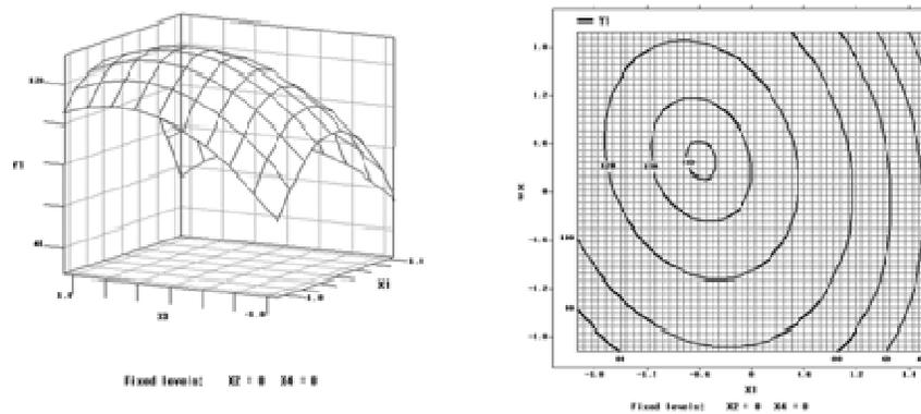
**Figure 5.** Response surface plot for L-LA production as a function of glucose ( $X_1$ ) and BE ( $X_3$ ) concentration while keeping peptone ( $X_2$ ) and YE ( $X_4$ ) at their respective zero level
