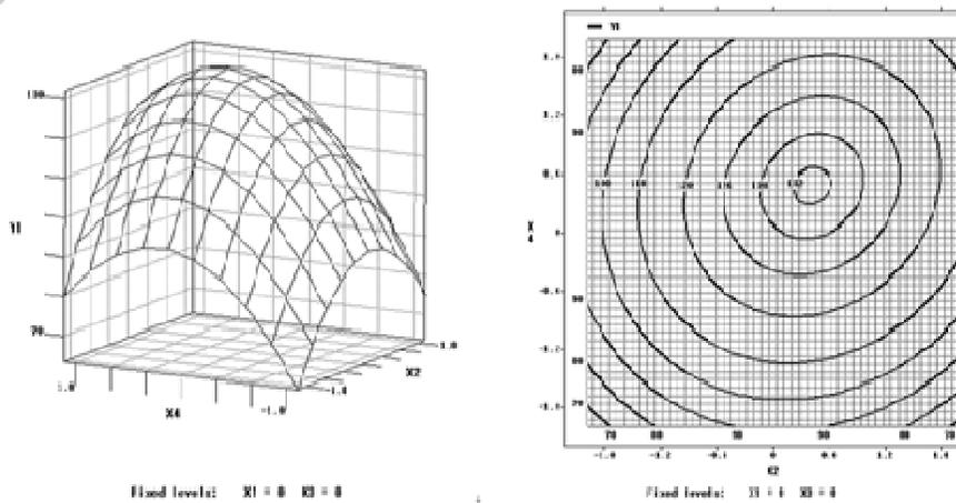
**Figure 8.** Response surface plot for L-LA production as a function of peptone ( $X_2$ ) and YE ( $X_4$ ) concentration while keeping glucose ( $X_1$ ) and BE ( $X_3$ ) at their respective zero level
