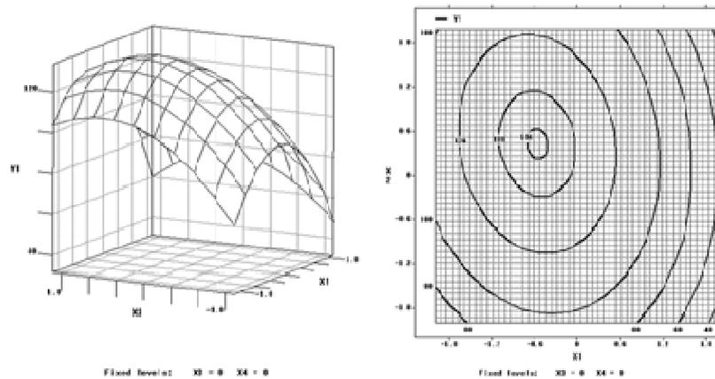
**Figure 4** Response surface plot for L-LA production as a function of glucose ( $X_1$ ) and peptone ( $X_2$ ) concentration while keeping BE ( $X_3$ ) and YE ( $X_4$ ) at their respective zero level
