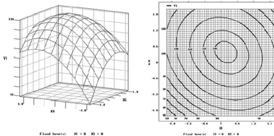
**Figure 9.** Response surface plot for L-LA production as a function of BE ( $X_3$ ) and YE ( $X_4$ ) concentration while keeping glucose ( $X_1$ ) and peptone ( $X_2$ ) at their respective zero level
