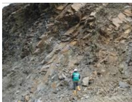
Figure 2 Fractured shale and phyllite.
