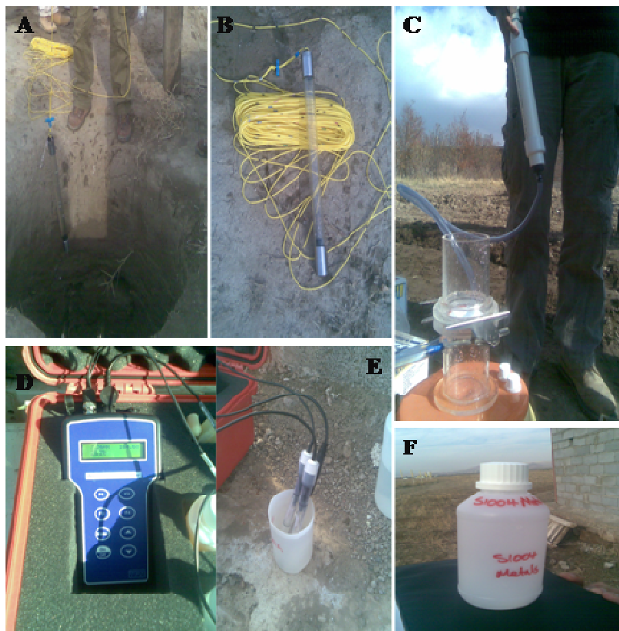
Figure 2 A, B) Water sampling; C) Filtering; F) storing and D, E) field analysis
