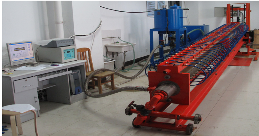
Figure 3. Photo of the gravel packing simulation equipment
