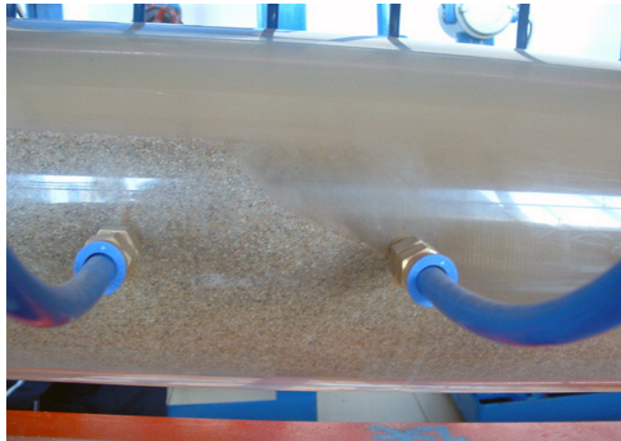
Figure 5. Image of \alpha wave sand-bed equilibrium height and packing front edge
