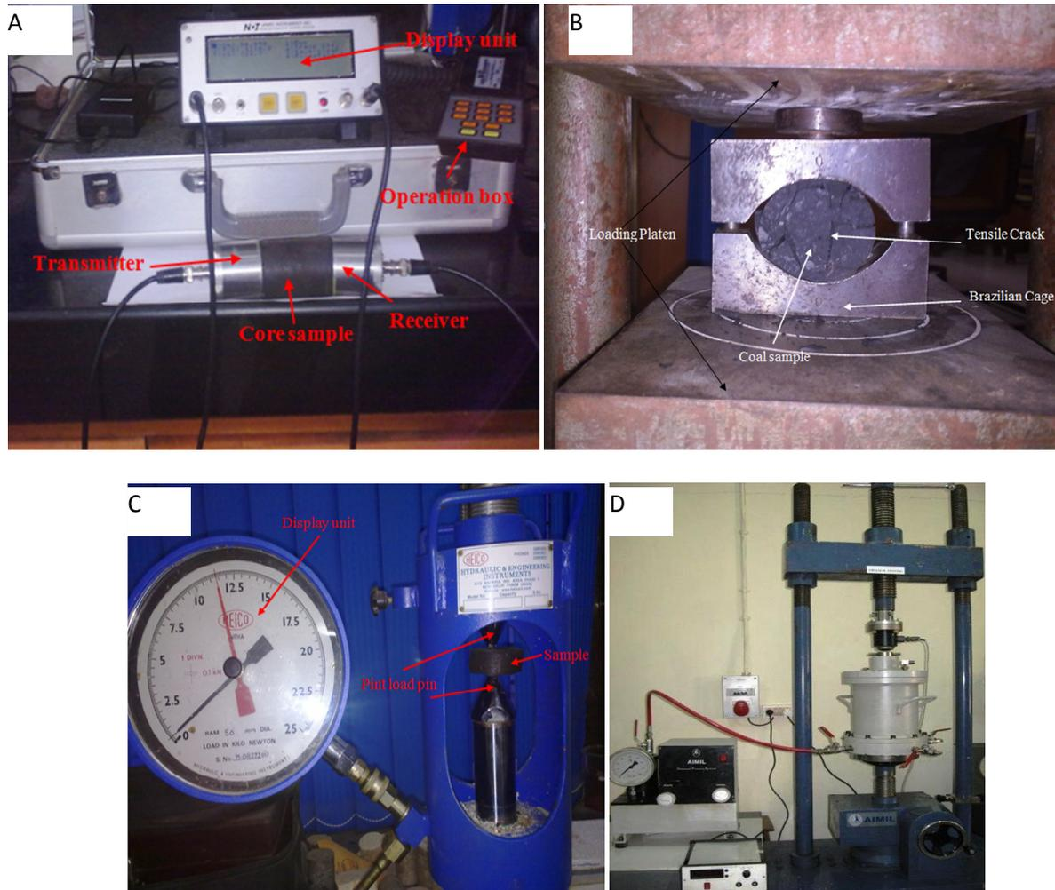
**Figure 2.** Measurement Instruments of geo-mechanical properties, A) P-wave velocity, B) Brazilian Test, C) Point Load Test, D) Triaxial Test.
