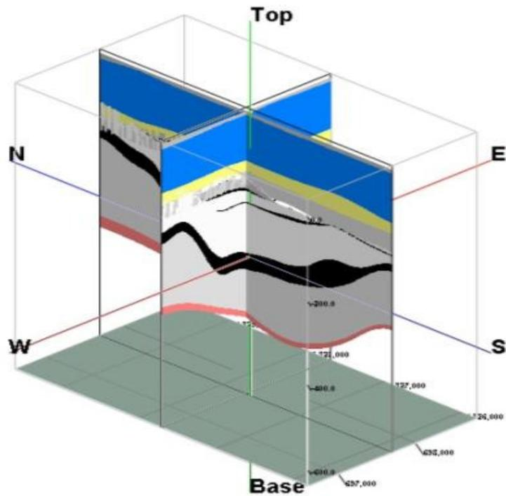
Figure8. The fence diagram, view of coal basin section as diagonally.
