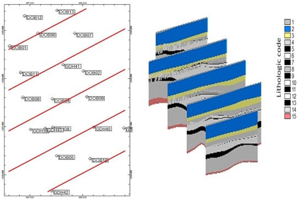
**Figure 6.** Fence diagram based on lithologic modelling-used Rockworks 15 with Inverse Distance (ID) algorithm for a grid size 50 m x 50 m x 20 m.
