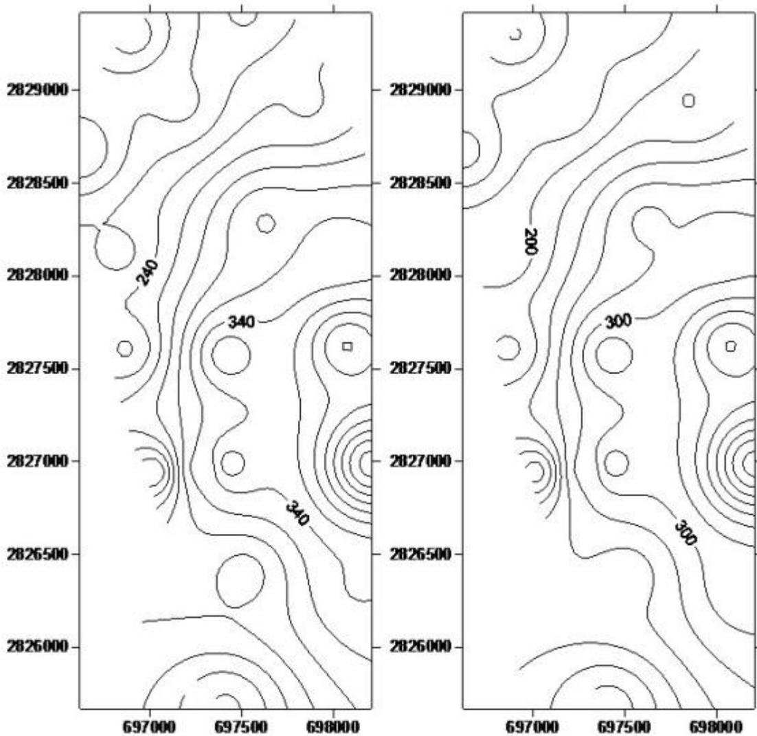
Figure12. Contour map of seam six using Surfer8 with Inverse Distance to a power (IDTP) algorithm in meter. Top surface shows in left and Base in right.
