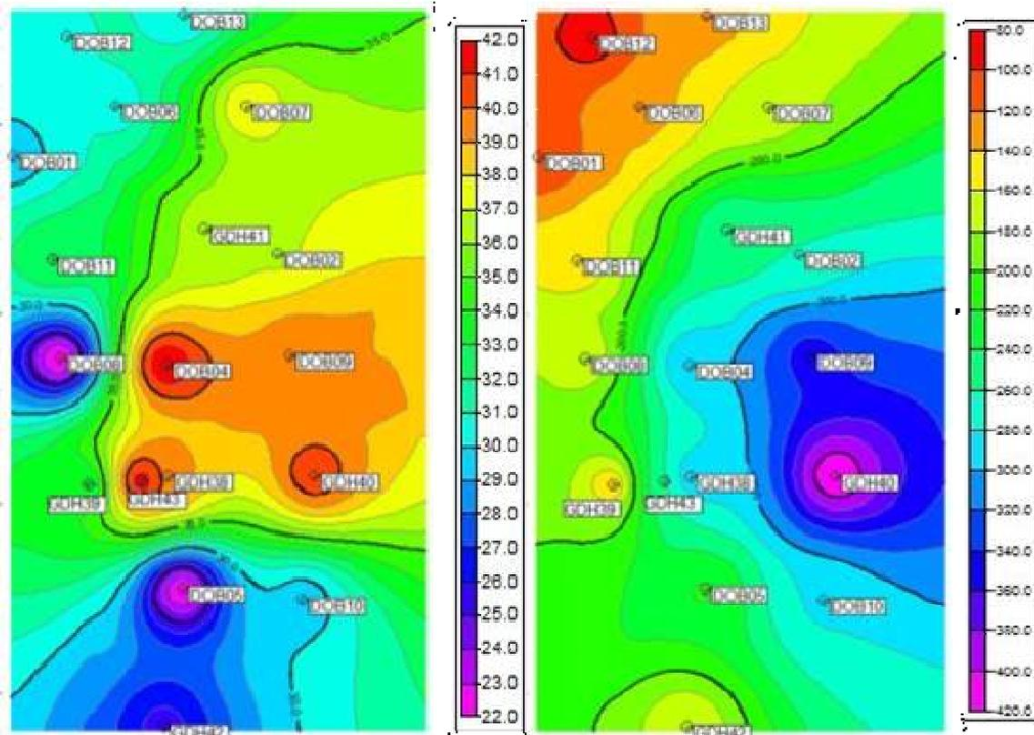
Figure9. The 2 dimensional map of coal seam VI-stratigraphic thickness (isopach map) in left side and Structural elevation in right.
