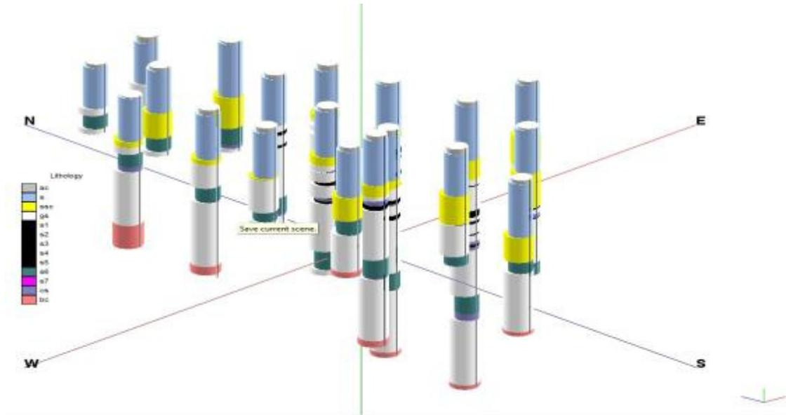
**Figure4.** All 18 logs are shown in a 3-D orientation. Here Lithologies are, ac=Alubium clay, S=Upper Dupitila sandstone formation, SSC=Lower Dupitila sandstone, silt, white clay formation, gs= Gondwana sand formation, s1=s2=s3.....=all are Coal seams, bc=Basement Complex.
