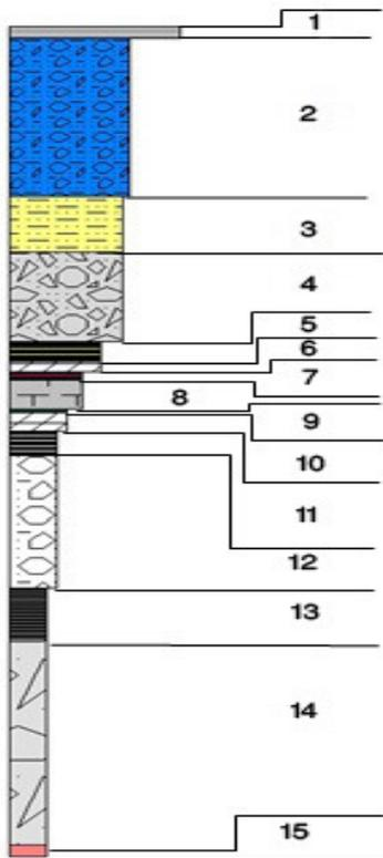
**Figure 5.** The 15 layers common data format for lithology analysis. The layers are, 1= Modhupur clay, 2= Upper Dupitila, 3= Lower Dupitila, 4= Sandstone, 5= Coal Seam II, 6=sandstone, 7=Coal seam III, 8= Sandstone, 9=Coal seam IV, 10=Sandstone, 11= Coal seam V, 12= Upper sandstone sequence of seam VI, 13= Coal seam VI, 14= Lower sandstone sequence of seam VI, 15= Basement complex. Seam I, coal+ shale are included in sandstone sequence for simplification.
